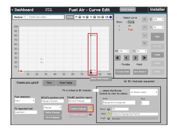
When Prepurge is confirmed, the SLATE Fuel Air Ratio reports that it is "At Prepurge" and this causes the SLATE Burner to measure the prepurge time.
