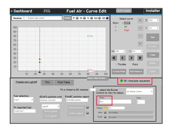
As an example, start by moving the throttled down to about 20%, select and move the air up to above the Fuel a bit to just make it different. (Normally this is done while watching a combustion analyzer.)
