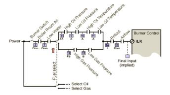
**11.** Under Annunciator Input Text, type in the desired name of each Analyzer Input string contact (T6-T19) in all of the strings used (refer to your application-specific wiring diagram). This function is not Analyzer specific; it's done at the Annunciator level so names can be written for all Analyzers (triggers) in this window. The following steps illustrate the dual path example provided in the image above.
