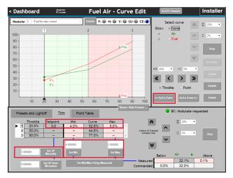
Next visit these two limits by using the trimmed actuator controls. Move the trimmed actuator up to Above limit (32 plus 5=37) and down the Below limit (32 minus 4 = 28). You'll have to stop right on the limiting value. The boxes should turn green.
