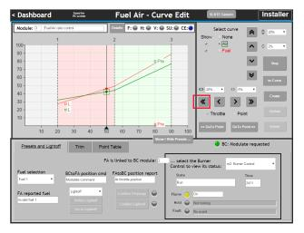
Adjust point 2. Select the second point, which means the actuators must stop very close to the point. There is a Go to Point button that allows the actuator to move to the point.
