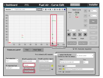
When the actuators have stopped the "Confirm Prepurge" button will become enabled. During commissioning, none of the steps occur automatically, the installer is always in control. Click the Confirm Prepurge button.
