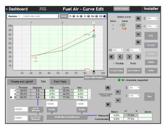
Note that all of the blue check mark circles are complete. The final step is to select the "Enable normal operation" in the Current Fuel Air Mode dropdown. Red lights will occur and the system will shut down. This is normal.
