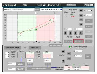
Set the Trim Setpoint to 2.0 by editing the box and clicking "Set SP Manually". This time, set the Min value using the other method. First move the trimmed actuator down until it's 2% below the curve, then click "Set Min/Max Using Measured". Notice that it turns green right away because it's already there.
