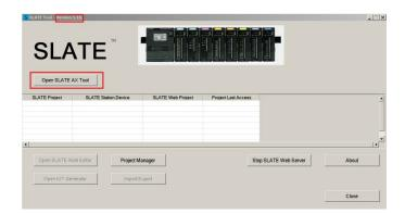
Honeywell will update the SLATE AX Tool periodically when new features are released. It is important to know what version you have installed and that information can be found in the upper left hand corner of the software.
