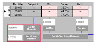
At each point, there must be a Min and a Max actuator deviation. These provide safety limits as a percent of actuator travel (e.g. the maximum amount it is allowed to deviate such as 5% or 2%. Both Min and Max are positive numbers. They are the magnitude of offset that is allowed)
