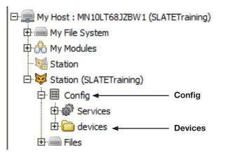
You will need to create a new device and put it in the devices folder. For the SLATE system you will see in the SLATE AX Tool Palette SLATEdevice. Click and drag the SLATEdevice from the Palette to the device folder in the Navigation pane until it is highlighted. Then drop it. See figure below.
