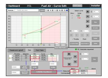
Set the Max value in the same way. Move the actuator up until it's 4% above the curve then click the "Set Min/Max Using Measured" button. When done, click "to Curve" to go back to the curve and unlock the throttle.
