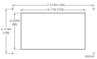
Mounting dimensions of color touch screen display in in. (mm).
