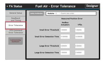
The VFD Command and Error Tolerance selection allows users to set small and large error tolerances with the VFD. To begin the Fuel Air Commissioning process Click the Commissioning Dashboard.
