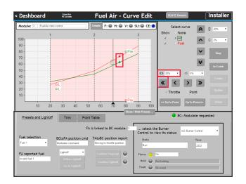
Jump up the throttle left by another 20% and note that as the actuators cross point 2, the segment turns green. It has been verified because all of it has been "visited". Normally this is done slowly while watching a gas analyzer, making any necessary adjustments, and creating new points as needed.
