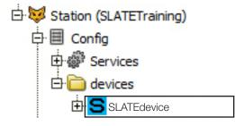
The SLATE AX Tool will require you to create a name for the new SLATE device within the devices folder. You can name the device
