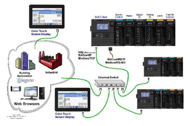
Fig. 1. 3 examples of SLATE devices.
