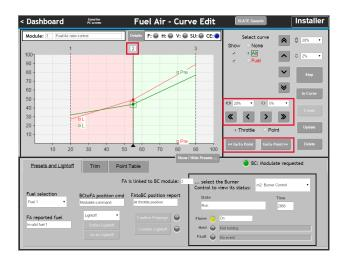
Select the fuel and move it up 5%. Not that the throttle gets locked and the fuel position is shown as an open circle when it stops. Both of these indicate it is off curve. Also not that Update is enabled. Click it to update point 2.
