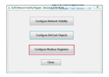
The same rule applies to Modbus registers as BACnet registers, a SLATE Wire Sheet with network inputs, network outputs, and registers must exist to show the registers on the configuration page. This view allows you to renumber the Register value (external) and edit the Register Name. Uncheck to exit the Protect Mode and enter your changes in the appropriate rows.
