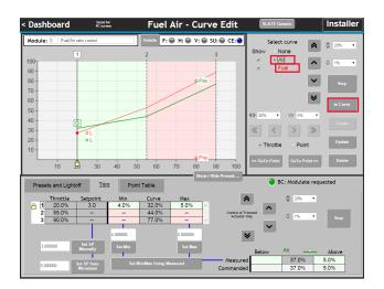
Use "Goto Point>>" to move the throttle to point 2. Again, normally this would be done slowly and one step at a time, while watching a gas analyzer.
