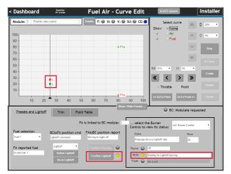
After Pilot and Main flame establishing periods have been completed, the SLATE Burner Control will be in the Run condition and will request modulation from the SLATE Fuel Air Ratio Control. It is now time to start building the Fuel/Air Curve.
