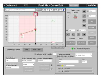
It is possible to move a selected point. Choose the "Point" radio button and move point 2 around to the left and right. Leave it at the 55% position.
