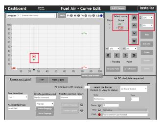
You will now need to define the Lightoff Preset by selecting "Lightoff" and clicking "Define Lightoff". Note that L appears next to these positions (below "None" has been chosen for the curve select to hide the selector box and show this more clearly).
