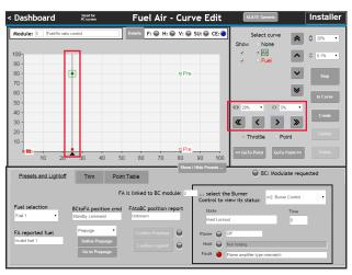
Next use the curve select and the up/down movement selectors and buttons to move the air actuator to about 20%, and the fuel actuator to about 25% (on the Y axis).
