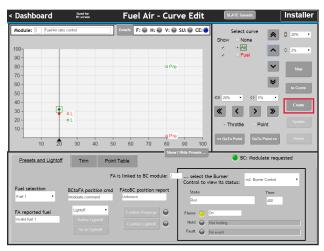
Point 1 now exits. (It is also selected because the throttle is close to the point, as shown by the box around the number.
