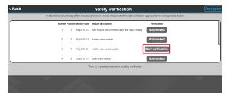
After the Safety Verification steps you will need to push the Reset button located on the Fuel Air Ratio module to complete the verification process. At this point you can go back to the Dashboard.
