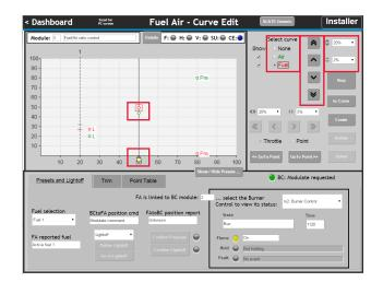
Point 2 now exists (and is selected). The curve segment between the points is pink colored because it has not been verified yet: there are ratios of fuel and air within the region that have not been visited and confirmed as OK. The throttle is unlocked because the actuators are now on-curve.
