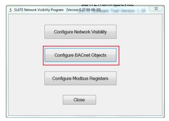
You can renumber the BACnet Object ID and Object Name. Uncheck to exit the Protect Mode and enter your changes in the appropriate rows.
