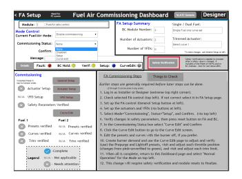
The Safety Verification screen will allow users to start the verification process. Click Start Verification button.
