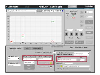
To send the SLATE Burner Control to the Prepurge position, select Prepurge in the drop down list and then click the "Go to Prepurge" button. The commanded position will move, and the actuators will move to the Prepurge position.
