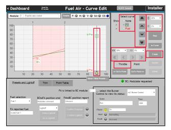
Now that a curve exists, actuators will follow it. Move the commanded throttle to the left by 20% and watch the actuators follow the curve to the new position. They are shown as "+" symbols while in motion.
