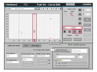
Select the Air and move it up to about 45% (y axis). Select the fuel and move it up to about 50%, above the air. Not that the throttle is locked (padlock icon) and the stopped actuator icons are circles instead of dots, indicating an off-curve condition. When done, click Create to create a second point.
